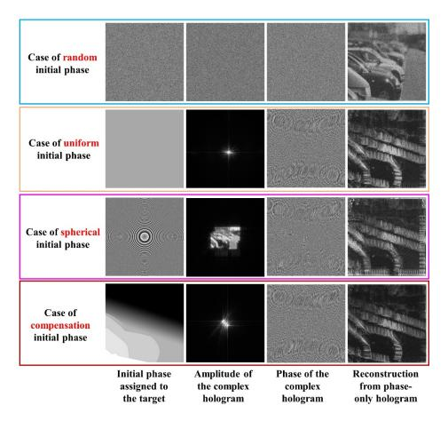
Fig. S2. Illustration of the influence of reconstruction from phase-only hologram by assigning different initial phase to the target object. The case of compensation initial phase is a smoothed phase distribution calculated according to the depth map.
