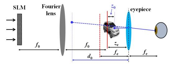
Fig. S1. Illustration of the calculation parameters involved in holographic near-eye display. The eyepiece magnifies the real holographic images into virtual contents that are perceived by the eye with accommodation cues.
